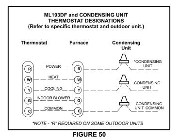
Install the room thermostat according to the instructions provided with the thermostat. See figure 50 for thermostat designations. If the furnace is being matched with a heat pump, refer to the FM21 installation instruction or appropriate dual fuel thermostat instructions.
