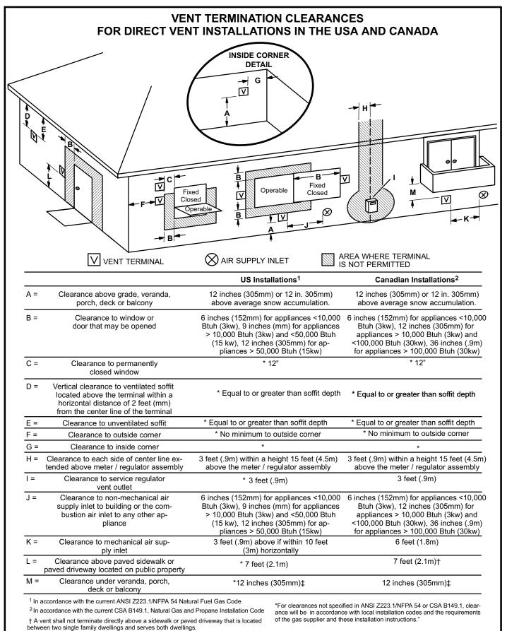
‡ Permitted only if veranda, porch, deck or balcony is fully open on a minimum of two sides beneath the floor. Lennox recommends avoiding this location if possible.
