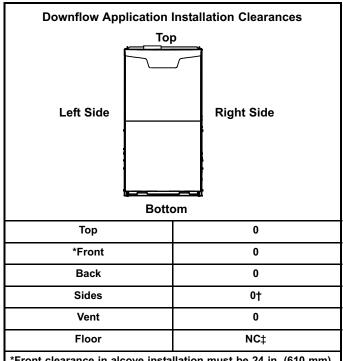
\*Front clearance in alcove installation must be 24 in. (610 mm). Maintain a minimum of 24 in. (610 mm) for front service access. †Allow proper clearances to accommodate condensate trap and vent pipe installation.
