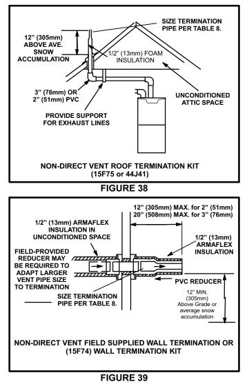
3 - If exhaust piping must be run up a side wall to position above snow accumulation or other obstructions, piping must be supported every 24 inches (610mm) as shown in figure 40. When exhaust piping must be run up an outside wall, any reduction in exhaust pipe size must be done after the final elbow.
