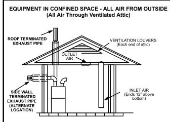
**NOTE**-The inlet and outlet air openings shall each have a free area of at least one square inch per 4,000 Btu (645mm<sup>2</sup> per 1.17kW) per hour of the total input rating of all equipment in the enclosure.
