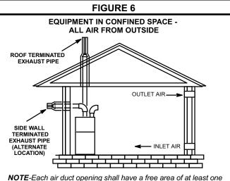
square inch per 2,000 Btu (645mm<sup>2</sup>per .59kW) per hour of the total input rating of all equipment in the enclosure. If the equipment room is located against an outside wall and the air openings communicate directly with the outdoors, each opening shall have a free area of at least 1 square inch per 4,000 Btu (645mm<sup>2</sup> per 1.17kW) per hour of the total input rating of all other equipment in the enclosure.
