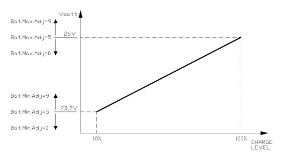
The Battery Charge detection follows this algorithm:
