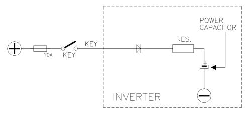
When the key is switched ON, the inverter tries to charge the power capacitors through a power resistance, and check if the capacitor are charged within a timeout. If they do not charge, an alarm is signalled; the
