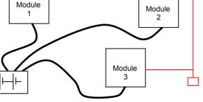
The red lines are can wires.
