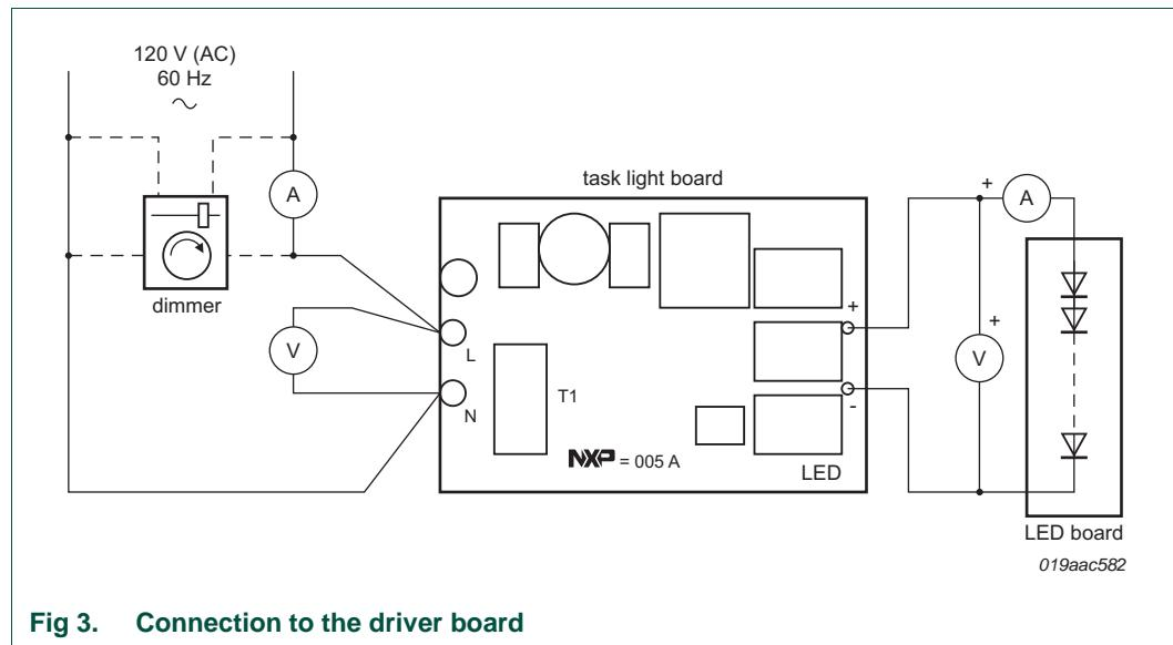
**Fig 3. Connection to the driver board**
