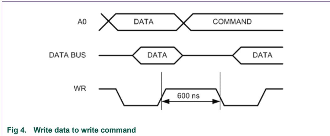
Fig 4. Write data to write command
