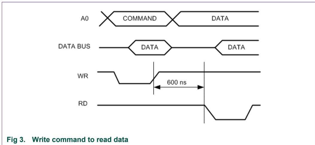
Fig 3. Write command to read data
