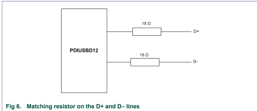
Fig 6. Matching resistor on the D+ and D- lines
