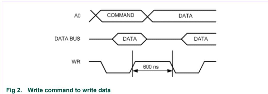
**Fig 2. Write command to write data**
