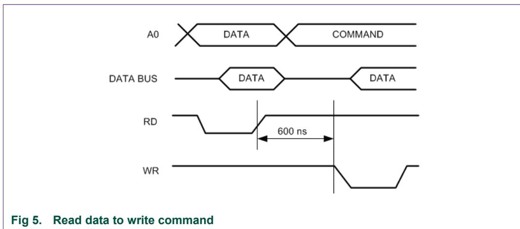
Fig 5. Read data to write command
