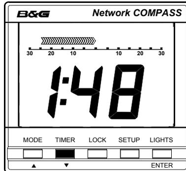
The timer can be set to any required value to a maximum time period of 99 hours 59 minutes. The analogue bar graph shows the time left, in minutes, from 30 minutes before time zero (bar graph on the left) to 30 minutes after (bar graph on the right).
