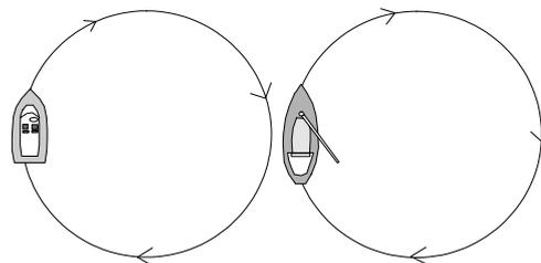
When the display shows a clockwise rotating segment press **ENTER** and turn the boat through a full circle
