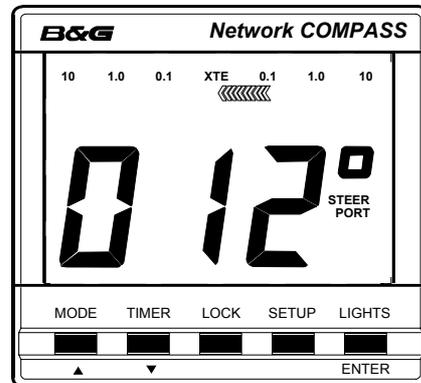
In this instance the vessel is heading starboard of the planned course. The display shows the current bearing and the **XTE** scale is visible above the bar graph which points to port. The legends **STEER** and **PORT** indicate the direction in which to steer to correct the error.
