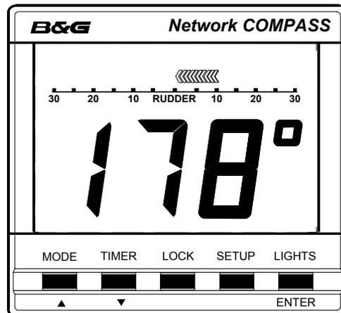
The vessel is turning to starboard, the display shows the current heading and the rudder scale is visible beneath the bar graph which points to port, the direction to turn the wheel to straighten the rudder.
