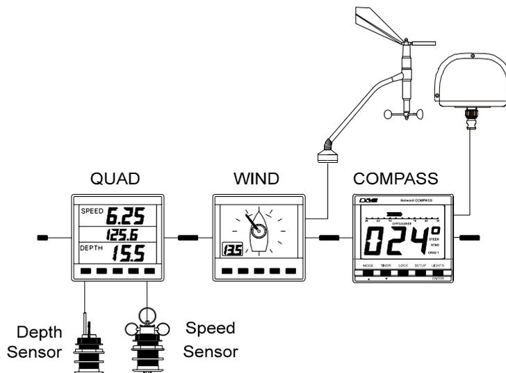
In this configuration the COMPASS unit is set to transducer mode and will send heading data to the other instruments. The other Network units are also transmitting data that the COMPASS may be able to use. For example, if the COMPASS is set to Head/Lift mode the wind angle data will cause it to switch between port and starboard tacks automatically.
