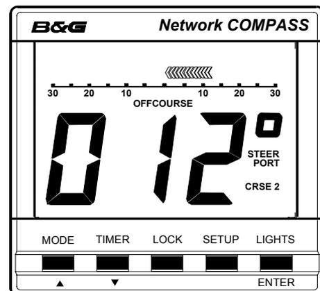
In this instance the vessel is heading starboard of the setting in the course 2 memory and the display shows the current bearing. The Off Course scale is visible below the bar graph which points to port, and the legends **STEER** and **PORT** indicate the direction in which to steer to correct the error.
