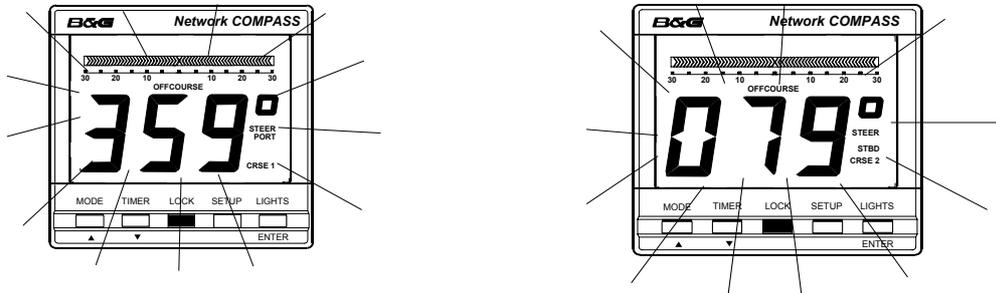
Pressing the **LOCK** key brings up the current course memory (e.g. **CRSE1**) which will flash on the display. Pressing **LOCK** twice displays the other course memory (**CRSE2**). Whilst the setting is displayed it can be adjusted by using the **▲** and **▼** keys (normally the **MODE** and **TIMER** keys). The display will revert to normal operation five seconds after the last key is pressed.
