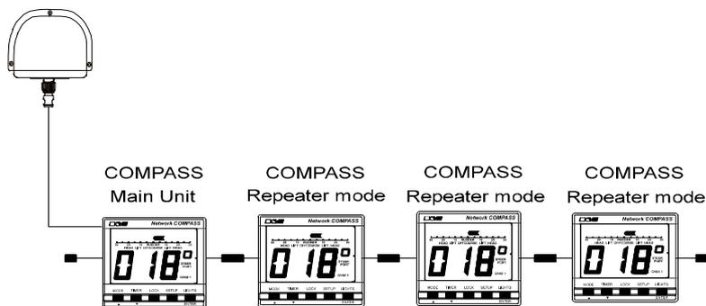
In this configuration the main unit controls all the measurement parameters such as offset and damping. These parameters can be changed via the keyboard on any of the units: repeaters will send appropriate network messages to the main unit so that it can keep its parameters up to date.
