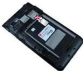
3. Insert the battery into place by aligning the gold contacts on the phone and the battery ❶ and press the battery down until it clicks into place ❷.
