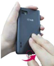
2. Insert the microSD card into the slot. Make sure the gold contact area is facing upwards.
