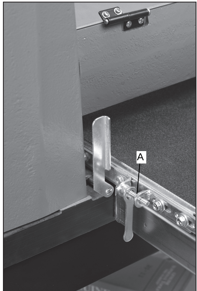
Fig. 9 Hanging wrench 1 of 2, for tracking conveyor
