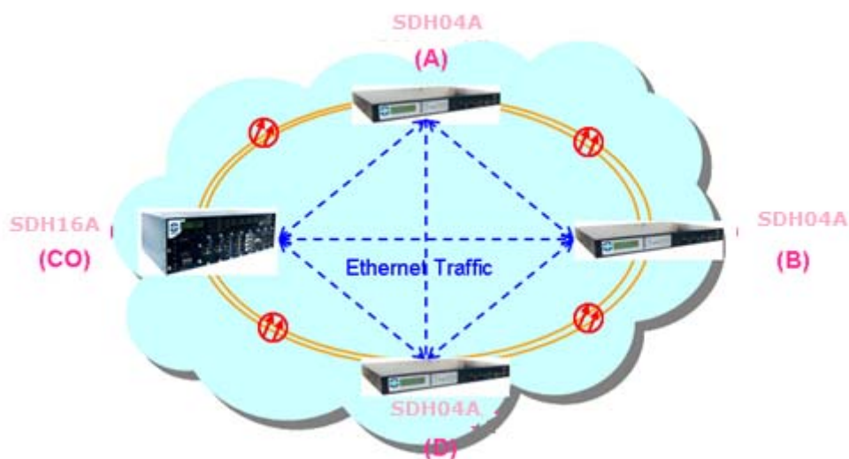
Figure 2-3 Fully Meshed E-LAN Service
