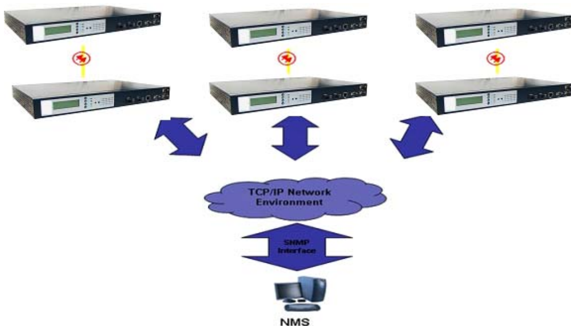
Figure 7-1 SNMP NMS structure
