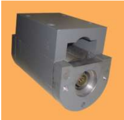
Detector probe with lead shielding arrangement for fixing onto 33 mm pipe lines
