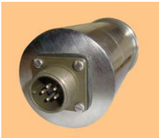
Detector probe with 5 pin MS connector (male)
