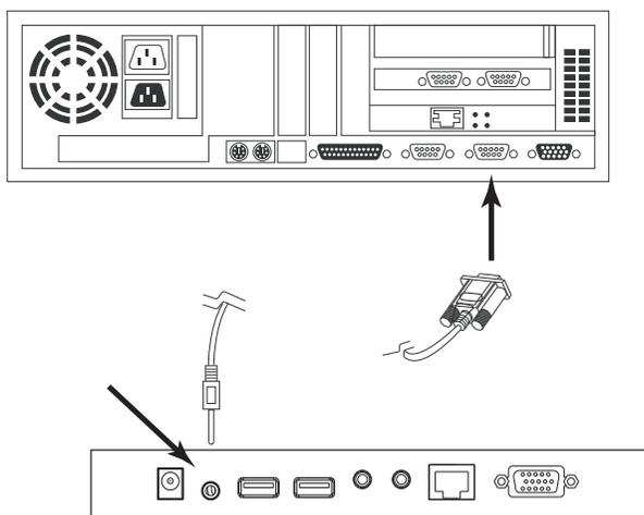
5. Make sure both units are connected by the Cat 5e cable, then plug in the Remote unit's power adapter.
