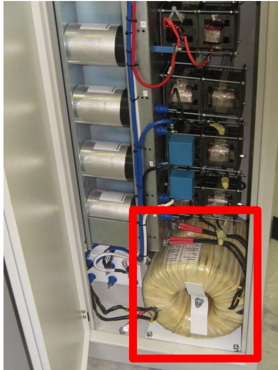
Figure 17: Position of the transformer in the DRI-10 enclosure.
