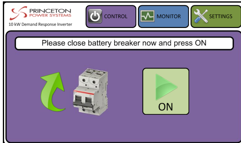
Figure 22: The DRI-10 Turn ON Confirmation screen.
