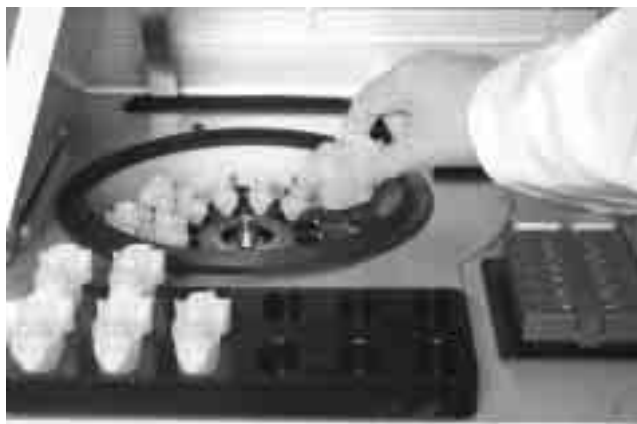
Figure 16 Load the assembled rotor adapters into the centrifuge buckets.
