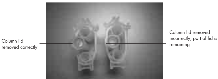
Figure 14 The PAXgene Shredder spin column is loaded into the middle position of the rotor adapter. Cut off the lid before loading the column.
