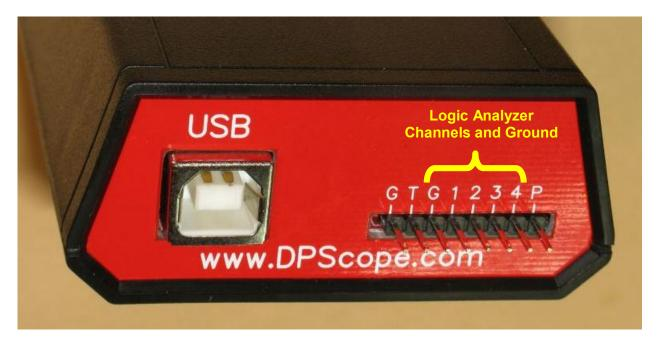
Otherwise this mode is very similar to the normal (real time) scope mode: You can trigger on each of the four channels, either on a rising or a falling edge, or have the acquisition in free running mode, and either single shot or repetitive capture. That said, the most common usage of a logic analyzer is in triggered, single shot mode . i.e. set up a trigger, wait for the trigger event to happen, capture one full record on all channels, then stop and analyze the data.
