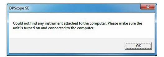
The DPScope SE should always be attached to a USB port directly at the computer, or through a <u>powered</u> USB hub. Unpowered USB hubs tend to have excessive supply voltage drop which needs to be compensated for (and which will reduce the scopes maximum voltage range). If in doubt you can check the actual USB supply voltage by selecting Utilities  $\rightarrow$  Check USB Supply. The nominal value is 5V but in reality can be as low as 4.3V.
