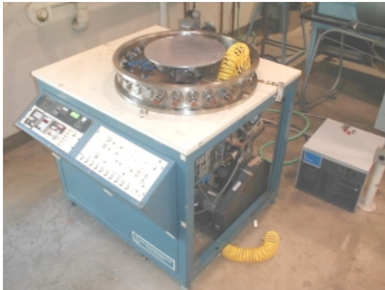
Figure 1. HVEC Vacuum Chamber Setup with Compressor (shown without belljar)
