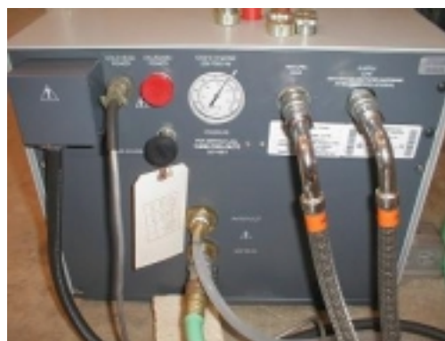
Figure 23. Cryopump Compressor Unit Helium Pressure Gauge
