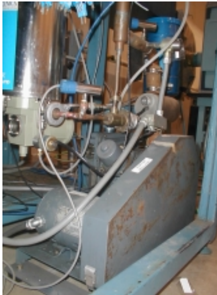
Figure 15. Roughing Pump Connected to Vacuum Chamber
