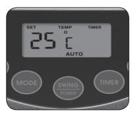
The LCD screen will display the default temperature of 25°C and will flash. When the temperature is flashing, you may set the desired temperature pressing the VARIABLE TEMPERATURE buttons on the control panel.
