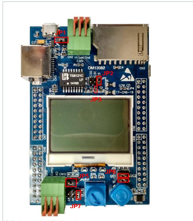
Fig 5. Jumper locations with default settings shown
