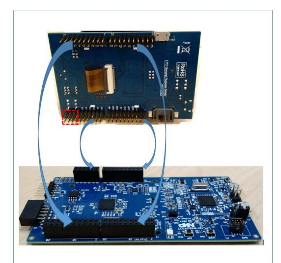
Fig 2. Installing the Shield on an LPCXpresso board (LPCXpresso4337 shown)
