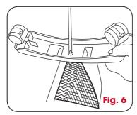
Turn the heater upright so that the wheels are holding up the heating unit.
