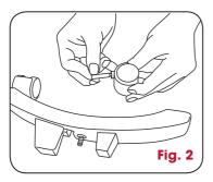
2. Line up the screw in the wheels with those in the base of the brackets, and secure.
