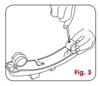
Turn the heater upside down. Place the plastic wheel brackets onto the two perforations, located at the base of the heater. Ensure the bracket with the centre hole (near the centre screw) is placed on the right hand side of the heater.
