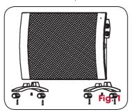
Insert the screw into the wheel, ensuring the flat end of the screw sits between the wheels.
