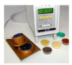
A professional laboratory instrument for precision measurements of  $a_w$  values (water activity) in foodstuffs and pharmaceutical products. The laboratory temperature should be maintained at a constant value, since the water activity depends on the temperature for many such products.
