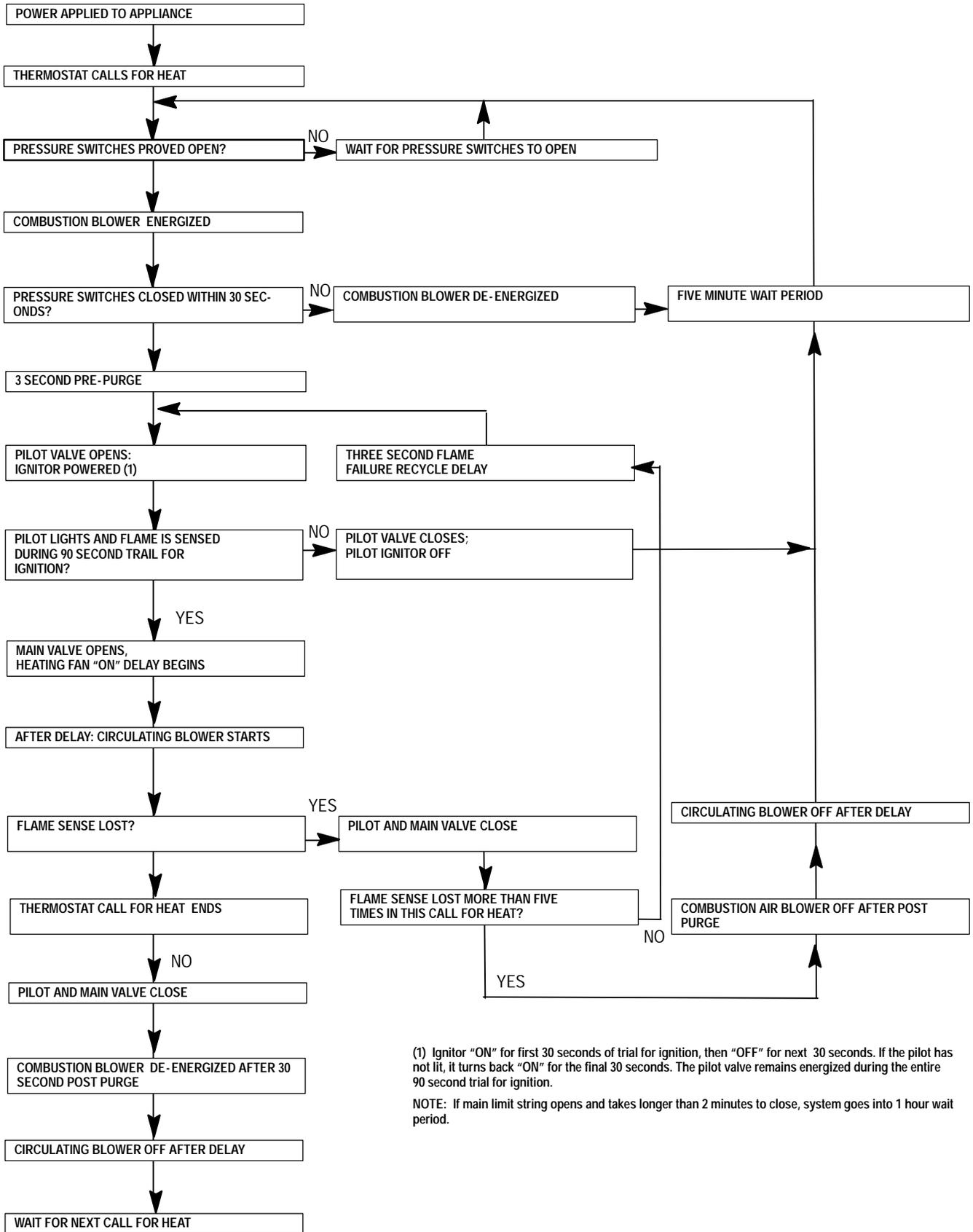
(1) Ignitor "ON" for first 30 seconds of trial for ignition, then "OFF" for next 30 seconds. If the pilot has not lit, it turns back "ON" for the final 30 seconds. The pilot valve remains energized during the entire 90 second trial for ignition.
