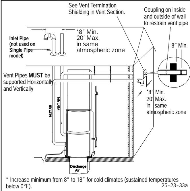
\* Increase minimum from 8" to 18" for cold climates (sustained temperatures below 0°F). 25-23-33a
