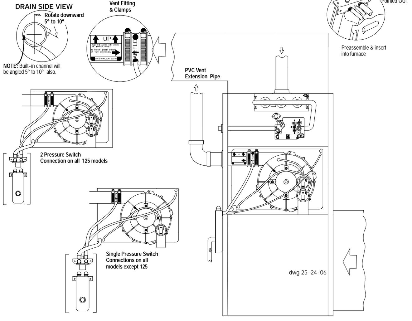
Upflow Installations - (Single Pipe & Direct Vent N9MP1 & N9MP2 Models) (See Figure 13)
