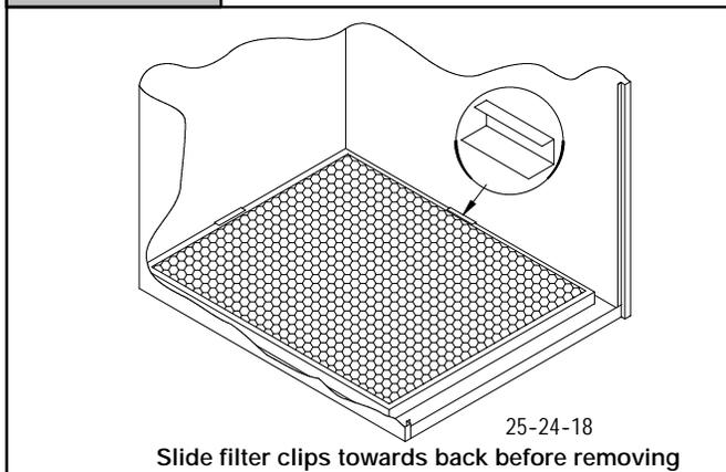
Refer to **Figure 36** and for guidelines to install filters. Furnaces which require larger filter media and have limited clearances on one side of furnace, require a standoff filter rack, see **Figure 36**, available from your distributor.
