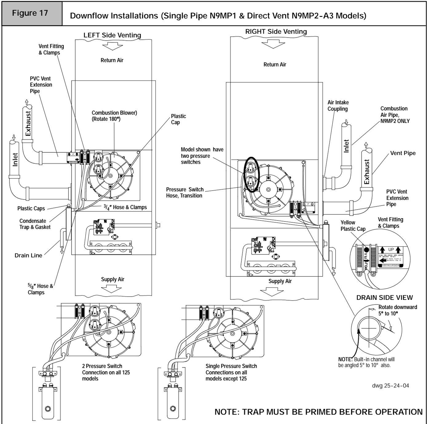
**Downflow Installations - (Single Pipe & Direct Vent N9MP1 & N9MP2 Models) (See Figure 17)**
