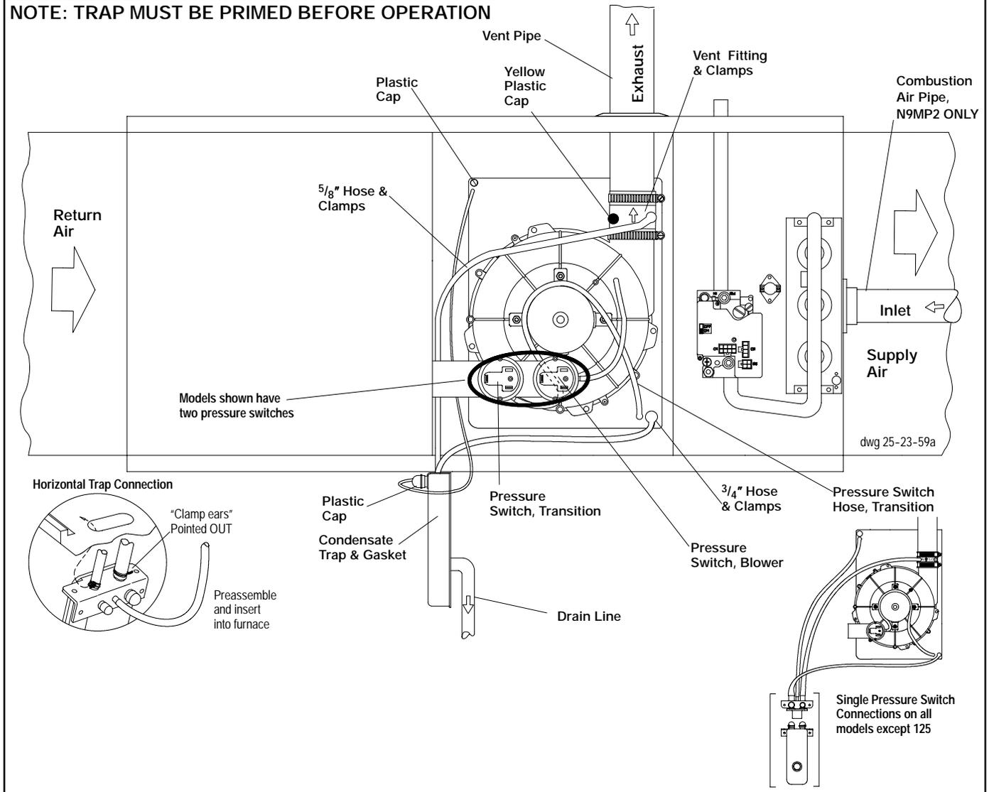
**Horizontal Right Installations - (Single Pipe & Direct Vent N9MP1 & N9MP2 Models) (See Figure 16)**
