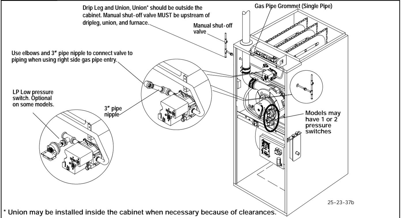
\* Union may be installed inside the cabinet when necessary because of clearances.
