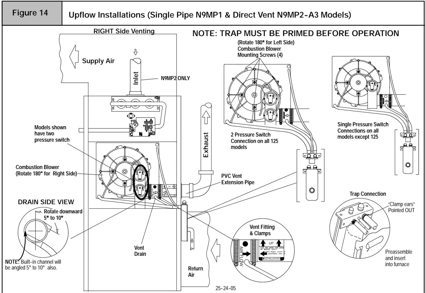
For left side or right side mounted condensate trap, the pressure tap on the condensate trap **MUST** be connected to the unused pressure tap located on the upper right hand corner of the plastic transition box. Remove the plastic caps from the pressure taps on the condensate trap and the plastic transition and connect with the  $\frac{5}{16}$ " OD rubber hose. (See **Figure 13** and **Figure 14**) Connect the  $\frac{5}{8}$ " OD rubber hose with the 90° bend to the lower
