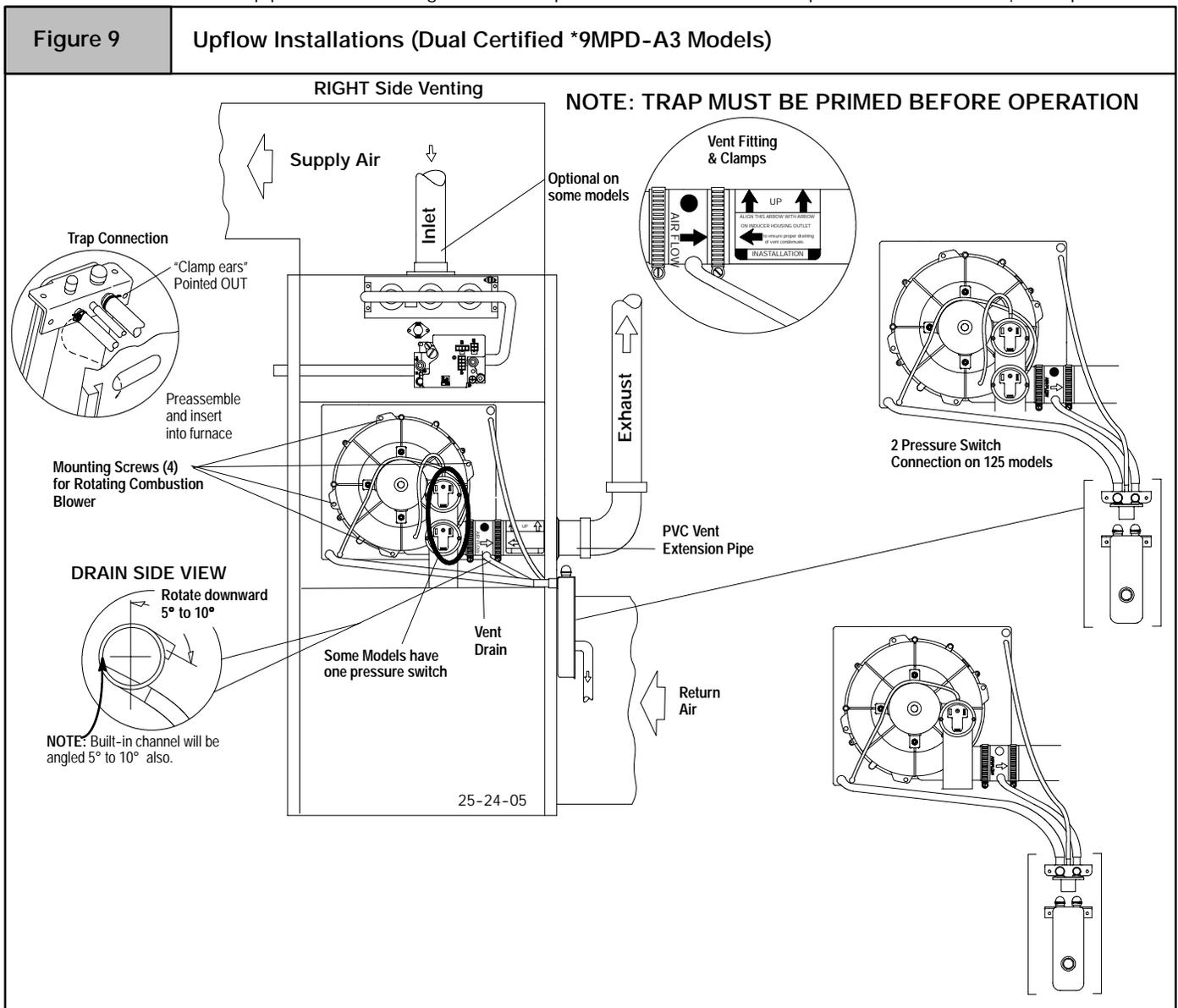
For left or right side mounted condensate trap, the pressure tap on the condensate trap **MUST** be connected to the unused pressure tap located on the upper right hand corner of the plastic
