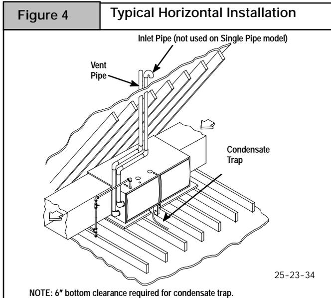
If the furnace is to be suspended from the floor joists in a crawl space or the rafters in an attic, it is necessary to use steel pipe straps or an angle iron frame to rigidly attach the furnace to prevent movement. These straps should be attached to the furnace with sheet metal screws and to the rafters or joists with bolts. The preferred method is to use an angle iron frame bolted to the rafters or joists. (Take caution to allow door panels to be removed for maintenance)
