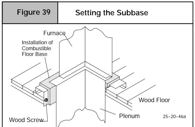
This subbase for combustible floors has been designed so that the height of the subbase raises the downflow coil off the floor to allow easy installation of the condensate drain. See **Figure 40**.
