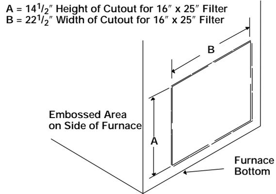
**NOTE:** Furnaces with 5 TONS cooling rating **require** two(2) side returns or one side return with bottom return.
