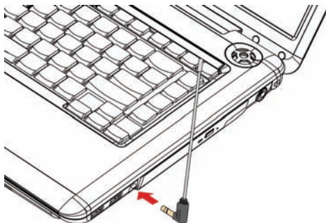
Figure 4-11 Connecting the FM tuner jack
