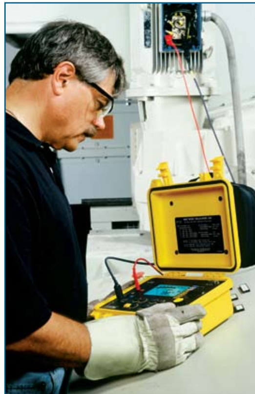
Large display and buttons make the Model 1060 ideal for shop use even with gloves.
