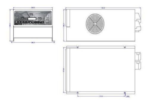
Dimension for Table Mounting/Horizontal SSL series 3000W PM-3000SSL-12/24
