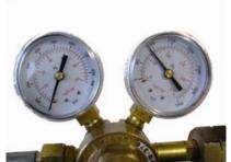
(5) Inspect the connections for leaks by applying some soap water on all connections (figures 12&13). If you notice bubbles
