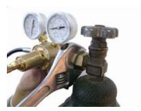
(3) Make sure the regulator inlet valve is closed. To close the regulator's valve, turn the regulator's adjusting knob in the counter clockwise direction.
