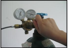
(6) Turn off the dual headed pressure regulator anti-clockwise until it is closed. At this time the lower pressure meter still indicates the pressure you charged the cartridge. Disconnect the HydroStik from the hydrogen cable. The meter will be back to 0.
