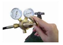
(9) Screw (clockwise) the HydroStik cartridge onto the SWAGELOK / Horizon adaptor assembly (figure 17).
