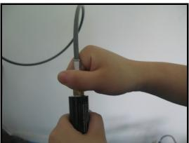
(7) Use the wrench to disconnect the hydrogen cable from the pressure regulator and turn the hydrogen supply off if not use them anymore.
