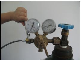
(3) Turn the duel headed pressure regulator handle anti-clockwise until it is tight. Make sure it is in the closed condition, so that the dual pressure regulator shows a zero reading on both dials.
