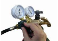
(8) Before connecting the HydroStik for filling, we must get rid of any non-Hydrogen gases from the system. Open (clockwise) the regulator's valve to 1 Bar (14.5PSI) for 5 secs and then close (counter-clockwise) it again (figure 16).
