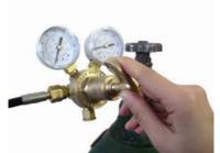
(4) Slowly open the compressed cylinder valve to observe the reading in the high pressure gauge (figure 8). This will indicate the internal pressure of the compressed cylinder, which should not be more than 200 Bar (2900PSI) (figure 10&11), but above 40 Bar (580 PSI).
