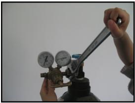
(2) Again using a wrench, screw the nut on the hydrogen cable provided to the dual headed pressure regulator provided. The nut needs to be tightened by turning the wrench anticlockwise. (See pictures below)
