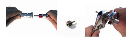
Insert the fine point of the special Horizon-designed adaptor (figure 2) into the male (QC4-D-200) part of the SWAGELOK connector. Once the adaptor component is positioned inside the SWAGELOK unit, use the wrench to tightly fasten the SWAGELOK nut onto the adaptor (figure 3). This will create a permanent connection between the adaptor and the male part of the SWAGELOK unit. Once the nut is fastened, do not attempt to disassemble it.
