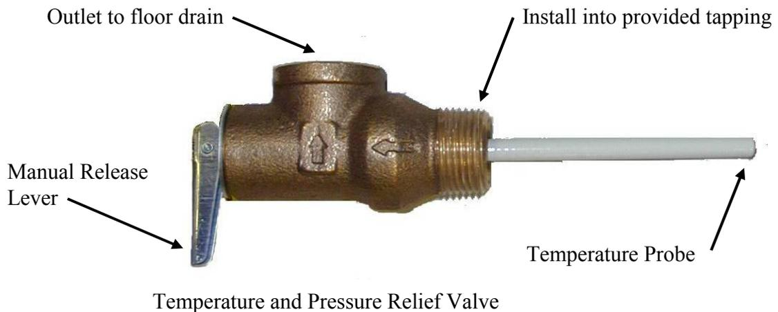
3. Install a relief valve overflow pipe to a nearby floor drain. CAUTION: No valve of any type should be installed between the relief valve and tank or in the drain line.
