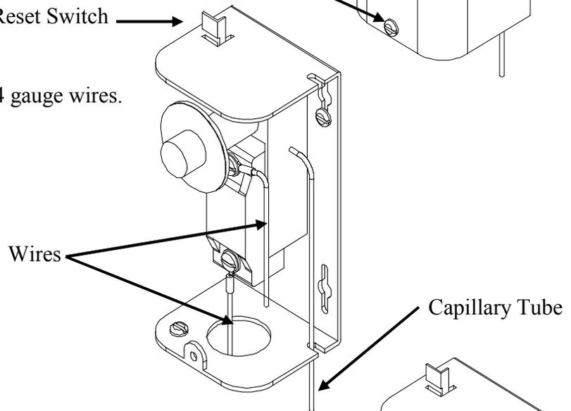
5. Remove capillary tube and bulb from thermowell
