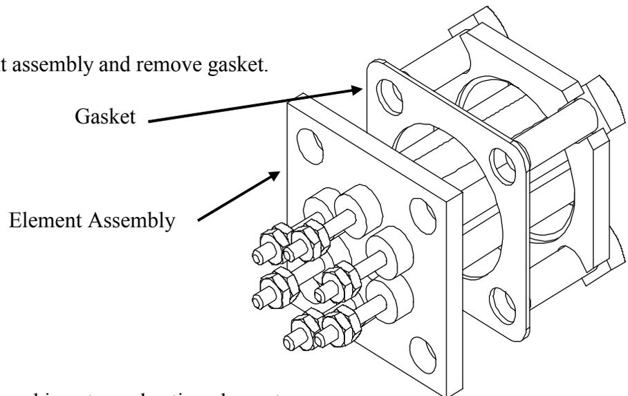
9. Install new gasket and insert new heating element.
