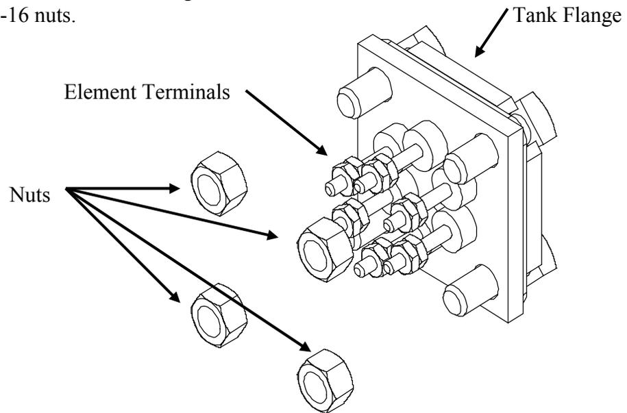
8. Withdraw element assembly and remove gasket.
