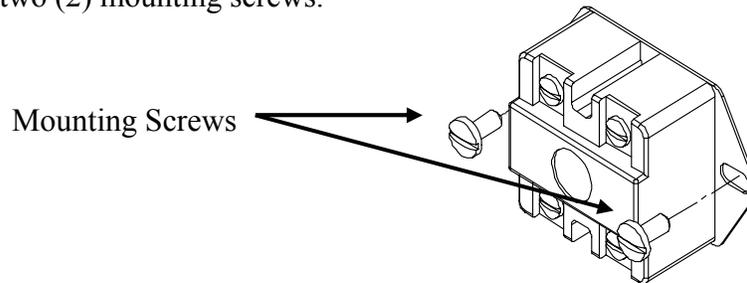
5. Replace control and install new high limit switch by performing above steps in reverse order. See wiring diagram included with drawing for assistance.
