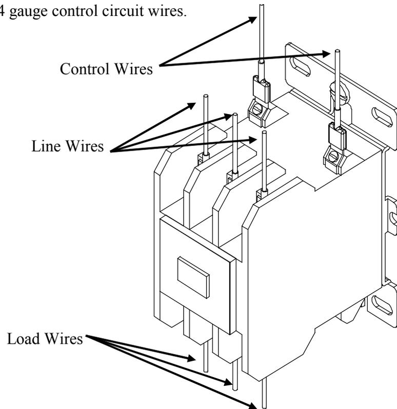
4. Loosen two (2) holding screws and remove contactor.
