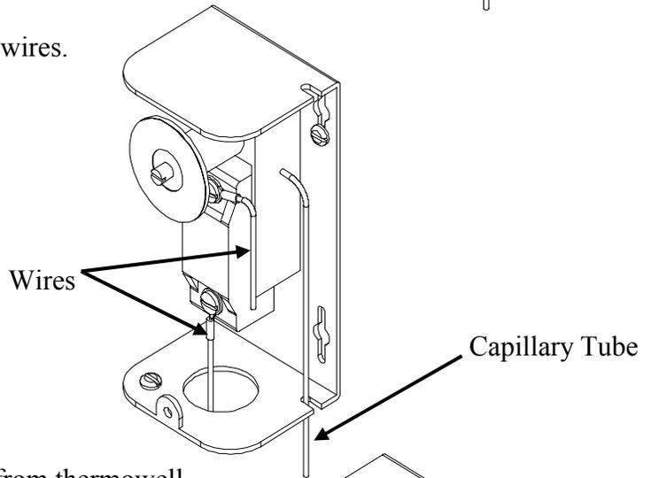
5. Remove capillary tube and bulb from thermowell.
