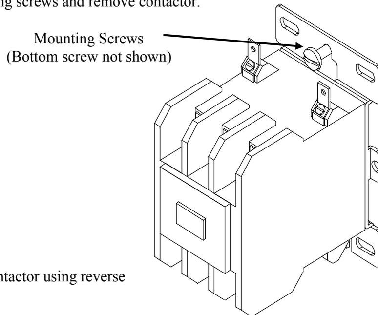
5. Replace with new contactor using reverse procedure.
