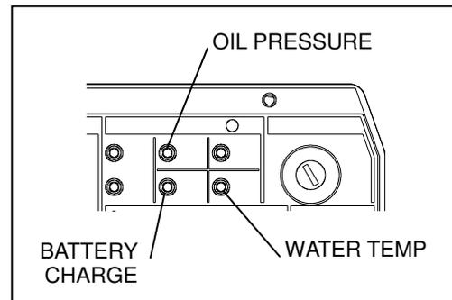
**(1) Coolant/Water Temperature Monitor Lamp**
