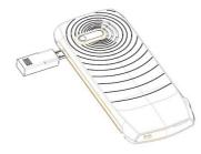
When charging, if the phone is switched on, the power quantity icon at the top right corner of the screen will twinkle and will stop twinkling and fully display when the battery is fully charged. If the phone is switch off, an icon will appear at the screen to show the battery is in charging.
