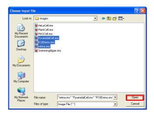
Select files for Batch execution and click on the Open. All selected files will be added to the Input list in Batch area.
