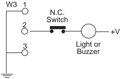
Figure 11-1—Example Watchdog Latch Circuit
