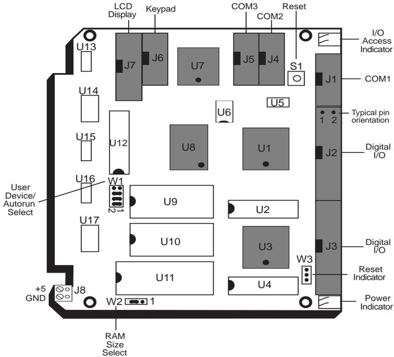
Figure 2-1—5082 Component Diagram
