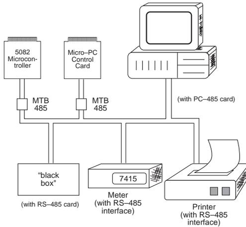
Figure 6-1—Multidrop Communications Network
