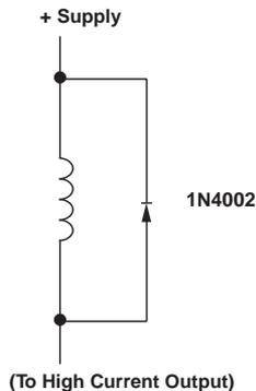
Figure 10-1 — Inductive Load Protection Circuitry
