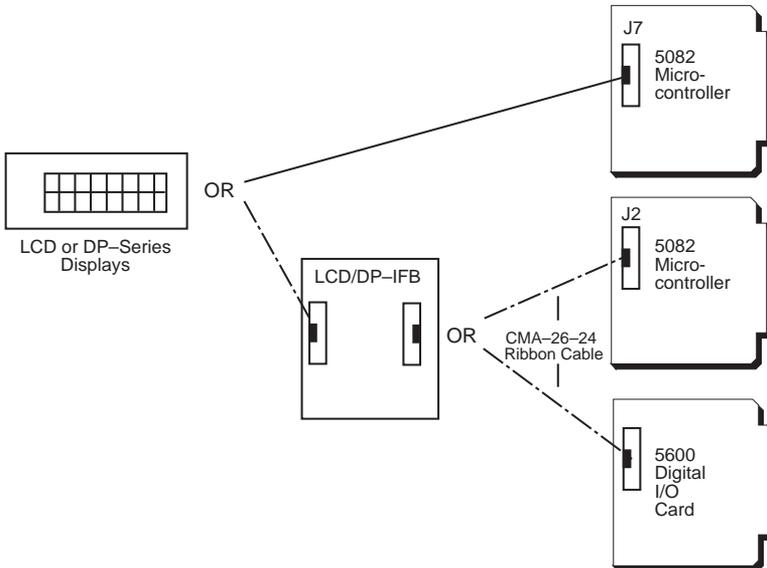
Figure 8-1—Display Configurations
