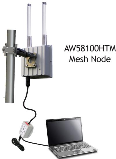
**Step 3.** The default IP address of the radio is written on its product label. This address is 192.168.88.11 with a subnet mask of 255.0.0.0. You must configure your PC's wired LAN port to the same subnet and an IP address different from that of the radio. With this configuration in place, you should be able to use a web browser on your PC to log in to the radio's interface.
