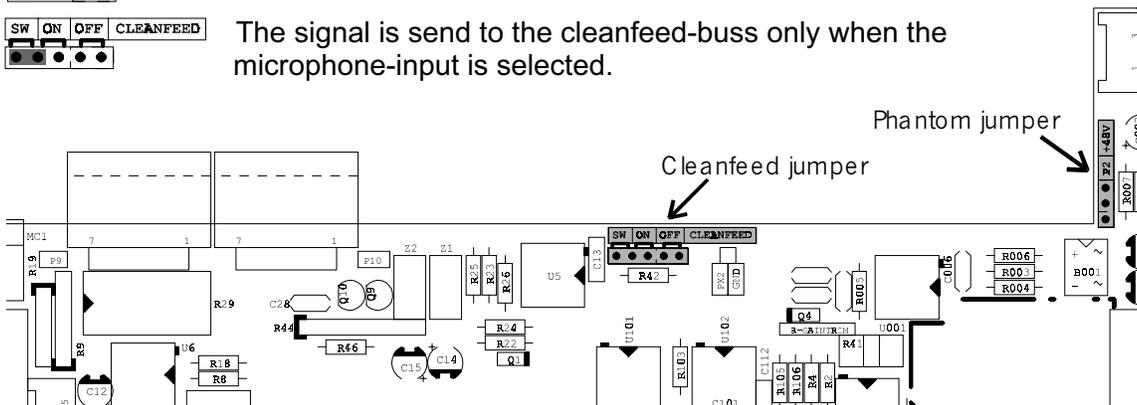
A phantom-power can be supplied to the microphone inputs. This can be done with the phantom-jumper (see the drawing above). By default the phantom-power is disabled on all the microphone inputs.
