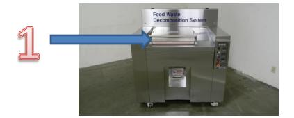
2. Lift open the top cover, and lift screen on left side.
