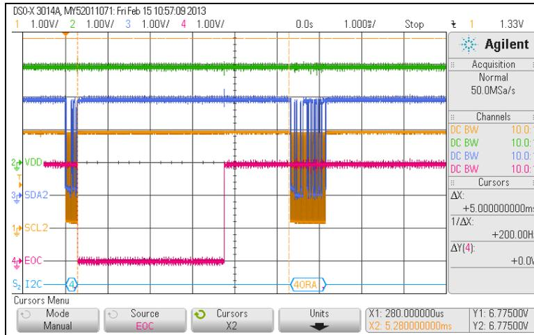
The simplest way to “detect” the end of a conversion (EOC) is to wait until the new data is definitely ready to read out. Being on the safe side; the conversion and the conditioning of the pressure and temperature value is completed after 6ms.
