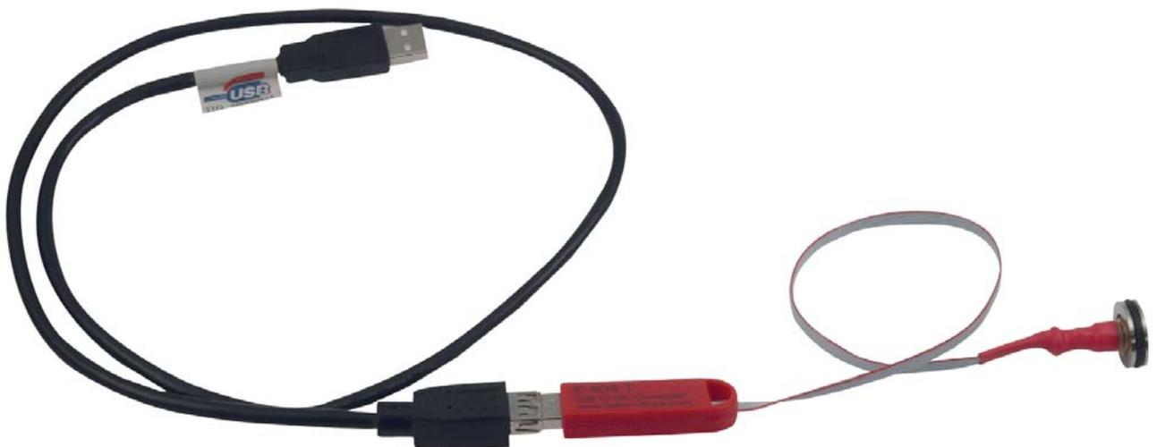
The K-404 converter is short circuit protected. The EOC-Pin is not connected and SDA and SCL are pulled up to the 3,3V supply by internal resistors. Please be careful by connection an oscilloscope with relation to earth because there is no galvanic isolation built in the converter.
