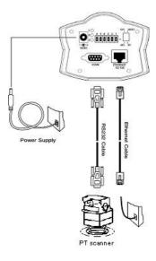
Shut down all the peripheral devices prior to connection. Connect the supplied cables from the IT210 Network Camera to related devices according to the above diagram. Note that the power adaptor must be kept unplugged until other cables are firmly connected.
