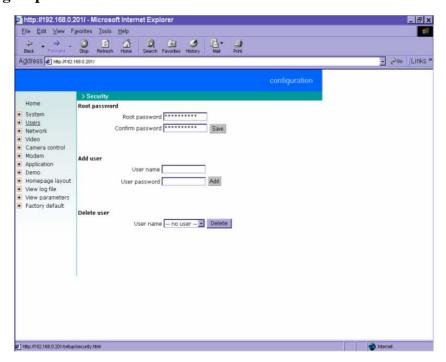
To change the administrator's password, type the new password in both text boxes identically. What is typed will be displayed as asterisks for security purposes. After pressing Save, the web browser will ask administrators for the new password for access.
