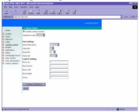
Since the IT210 Network Camera can be used in either PPP network or Ethernet network, the single serial port can control either external serial port devices like camera positioning devices or a data modem. While in PPP interface, go to Modem page for modem configuration. Options on this page will be ignored.
