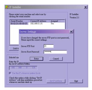
Once installation is complete, administrators should follow the actions in the "First access to the IT210 Network Camera" section for necessary checks and configurations. Experienced administrators may use the customized config.ini script file to perform a quick setup via FTP. Detailed procedure can be found on the section "One-shot fast configuration via FTP".
