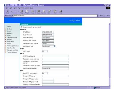
Any change made to this page will make the system restart to validate. Make sure every field is correctly typed before clicking on Save.
