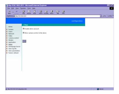
To setup the IT210 Network Camera for demonstration to the public, administrators need to choose service(s) to be opened. After checking "Enable demo account", user may use "demo" as general user name and password is not required. Regarding to the demo user account, "Allow camera control while demo" can be limited to differ from managed users. That will prevent demo user account from interfering with the normal operations.
