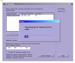
If the IP is not taken by another network device in the network, the Installer program will continue with the setup. Otherwise another message window will warn that the assigned IP conflicts. In this case, administrators should ask the network supervisor for a vacant IP address.
