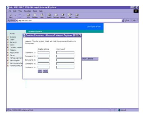
To enter more commands or commands other than pan and tilt, a flexible URL is provided for customized interface. See the "Clear data path for proprietary commands" section in Advanced functions for details.
