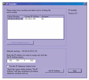
If the administrator wants to fix the IP address of the unit, check the option "Use this IP whenever system boots" to skip future installation procedures. Otherwise the unit will need installation whenever it restarts.
