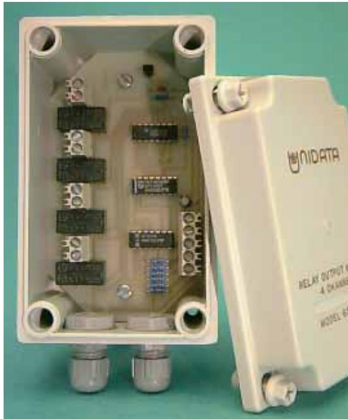
*Model 6525A 4-Channel Relay Control Module*
