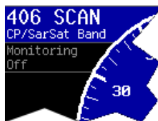
Fig. 18 Display of Cospas-Sarsat Scanning-Mode
