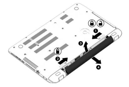
Reverse this procedure to install the battery.
