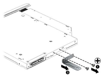
Reverse this procedure to reassemble and install the optical drive.
