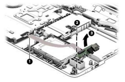
Reverse this procedure to install the USB board and cables.
