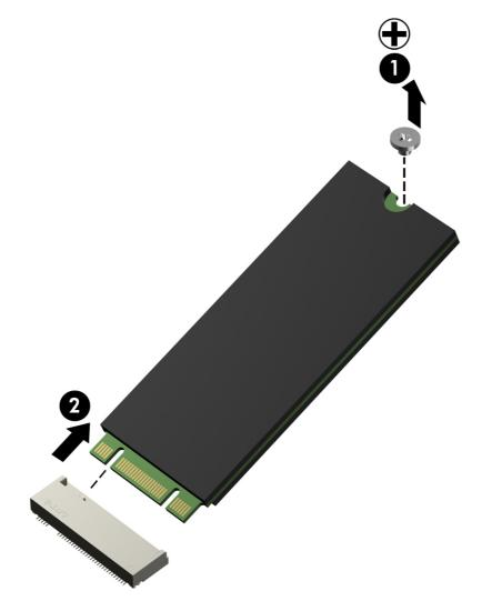
Reverse this procedure to install the solid-state drive.
