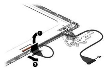
12. If it is necessary to replace the webcamera/microphone perform the following: Lift the module (1) from the adhesive holding it in place on the display bezel and disconnect the module connector (2) if you have not already done so when removing the display cable.
