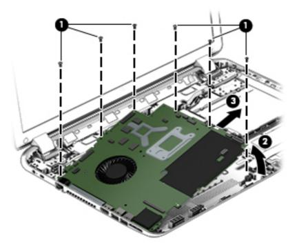
6. Turn the system board over and remove the solid sate drive before replacing the system board.
