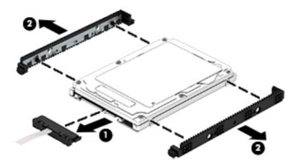
Reverse these procedures to reassemble and install the hard drive.
