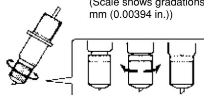
\* One full rotation moves the blade 0.5 mm (0.0197 in.) up or down. (Scale shows gradations of 0.1 mm (0.00394 in.))
