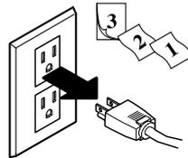
**NOTICE** Do not switch off the main power while printing is in progress. Doing so causes the printing head to remain in contact with the sheet, which may damage the head.
