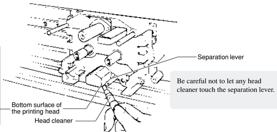
If this cleaning fails to remove all grime, then use the included head-cleaning sheet to perform cleaning.
