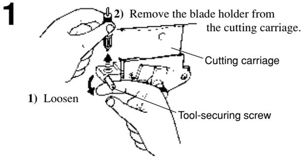
Leave the tool-securing screw loose. Tightening the screw makes it more difficult to install the blade holder.
