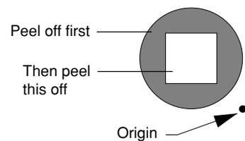
Use the tool force control slider to adjust the blade force so that results like those shown above are not obtained. Gradually increase the cutter force until you reach the optimum level.
