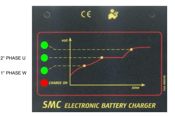
The charging cycle is divided in 2 phases (with reference to the front panel of the charger).
