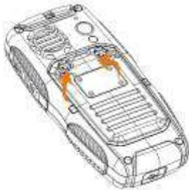
3. Confirm the battery is correctly installed before powering on.
