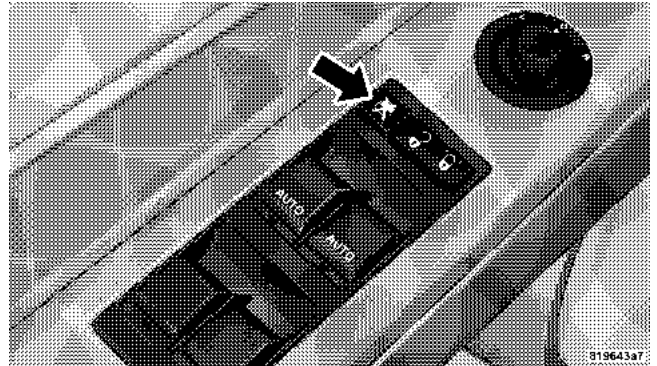
Window Lockout Switch
