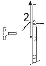
3- Lock in place using the ball lock pin.
