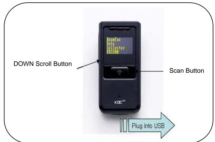
Figure 6 - Reset Function for KDC200 - KDC200P - KDC300
