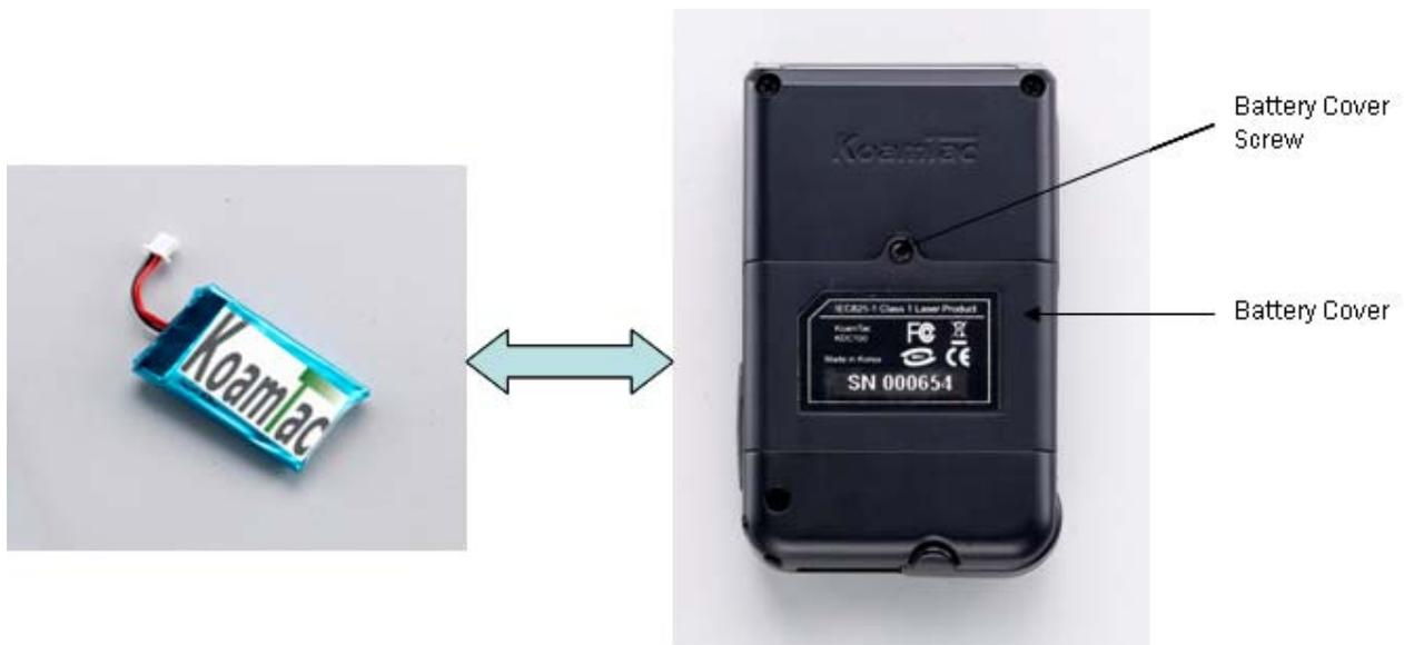
Figure 8 - Replacing KDC Battery
