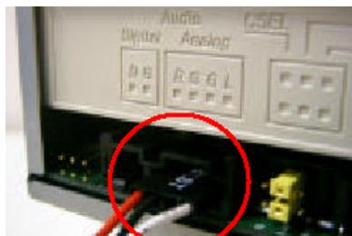
If you have a sound card or an audio interface card, use the audio cable to connect from the sound card audio port to the CD-ReWritable drive's analog audio out connector located on the back panel.
