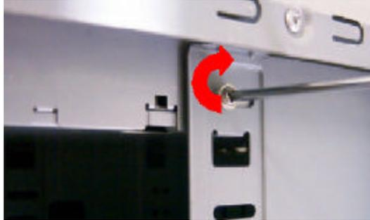
Secure the drive using four screws included in the accessory pack.
