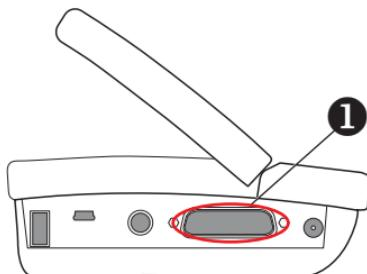
Connect a pyroelectric sensor to the 25-pin connector and turn the meter ON. Note: Contact Coherent if the sensor has a BNC plug and did not ship with a 25-pin adapter (refer to the "Calibration and Warranty" section of the User manual for contact information).
