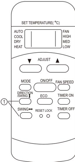
1. For RG51Q/BG(C)E models, when press the DIRECTION/SWING(↑↓) button, the louver changes 6 degree in angle for each press. If keep pushing more than 2 seconds, the louver will swing up and down automatically. Press the SWING(↔) button, the vertical louver will swing left and right automatically.
