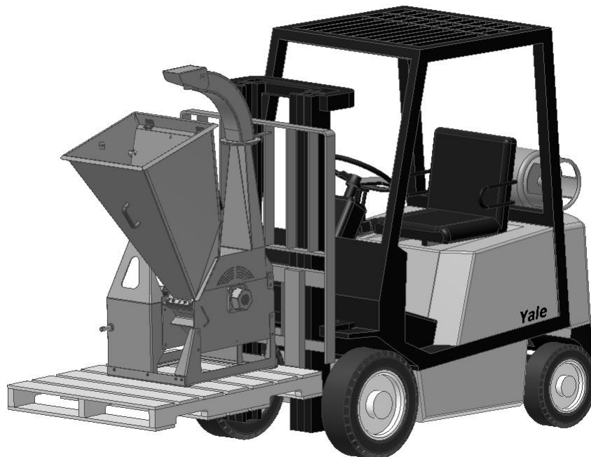
Figure 3 Lifting with fork lift truck, PTO
