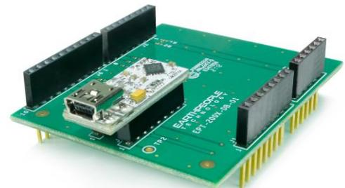
Mini B cable into the board connector and an open USB port on the PC. When the board is connected the USB driver (described in the previous section) automatically loads.
