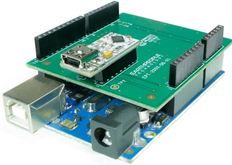
Connect the Uno to the PC using a USB Cable.
