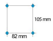
Attach both brackets to the wall using suitable hardware and align using the spirit level.
