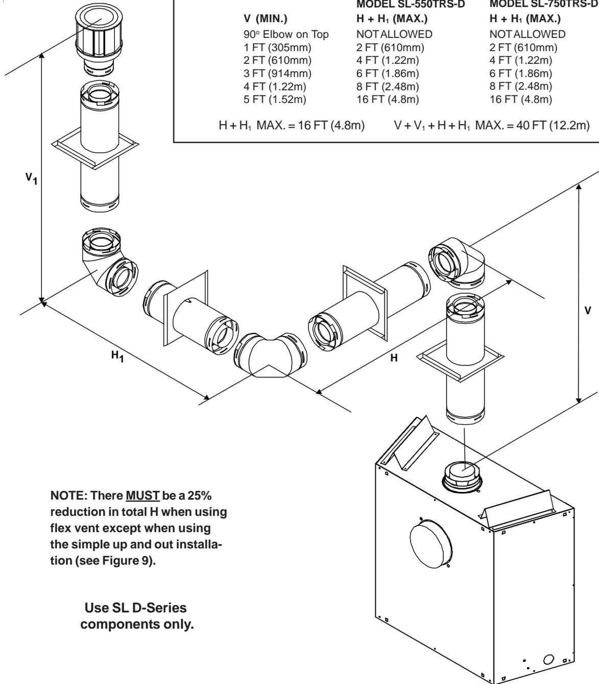
**NOTE:** There **MUST** be a 25% reduction in total H when using flex vent except when using the simple up and out installation (see Figure 9).
