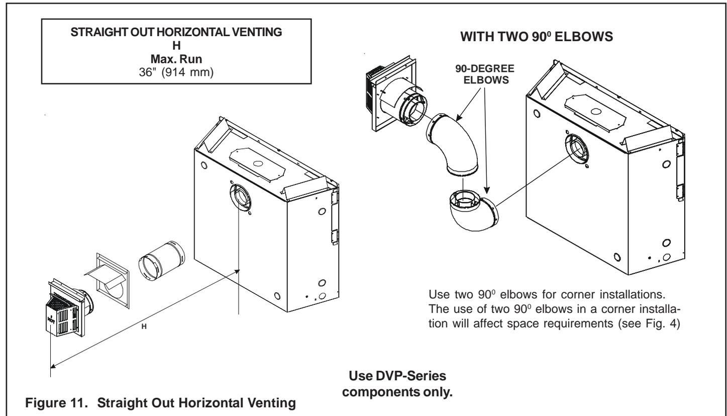
Figure 11. Straight Out Horizontal Venting
