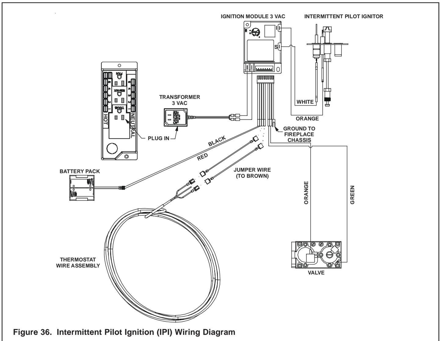
**Figure 36. Intermittent Pilot Ignition (IPI) Wiring Diagram**
