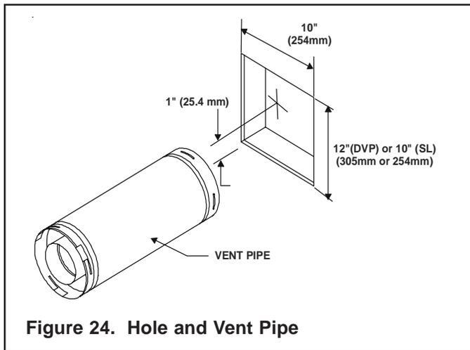
**Figure 24. Hole and Vent Pipe**
