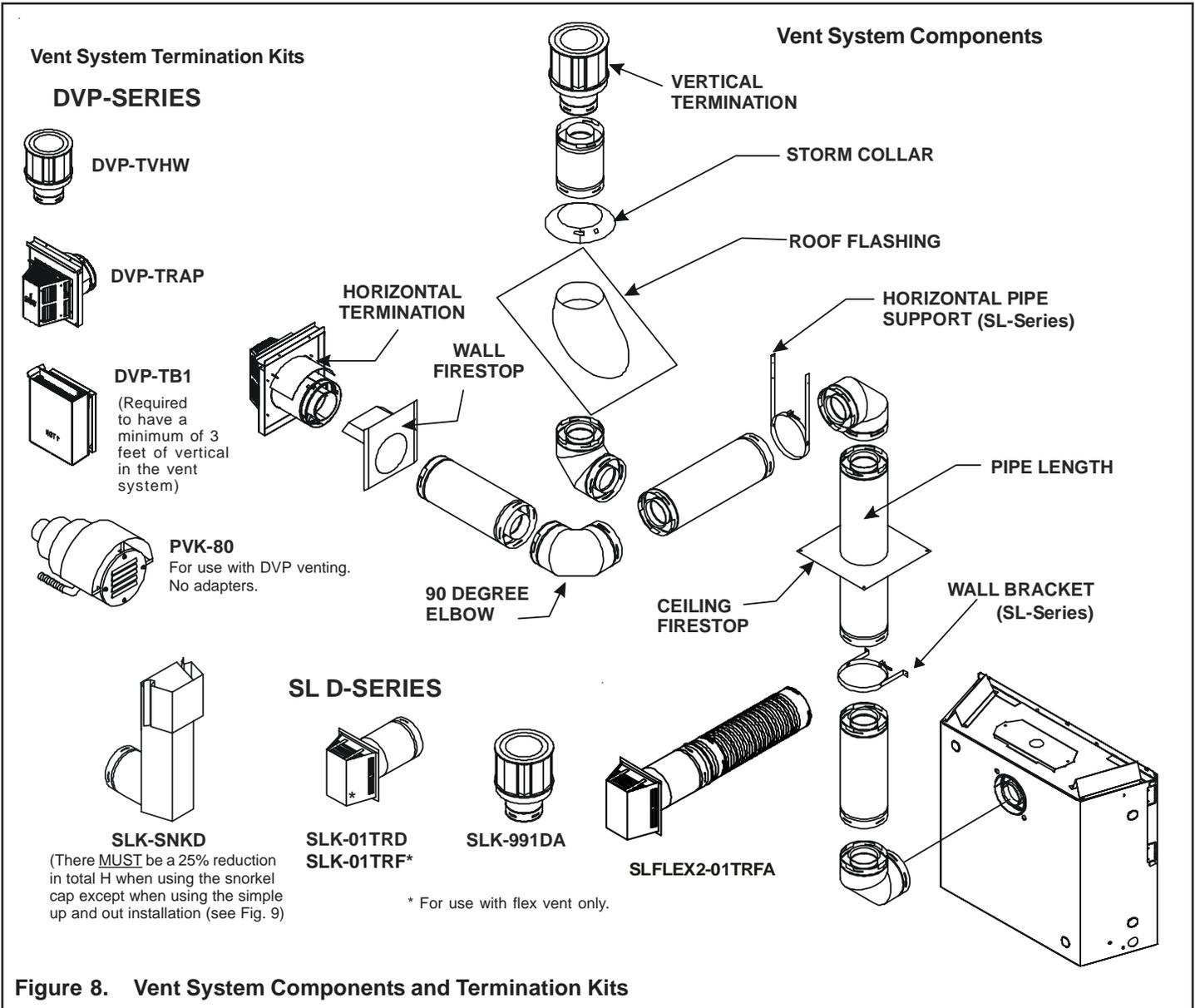
**Figure 8. Vent System Components and Termination Kits**
