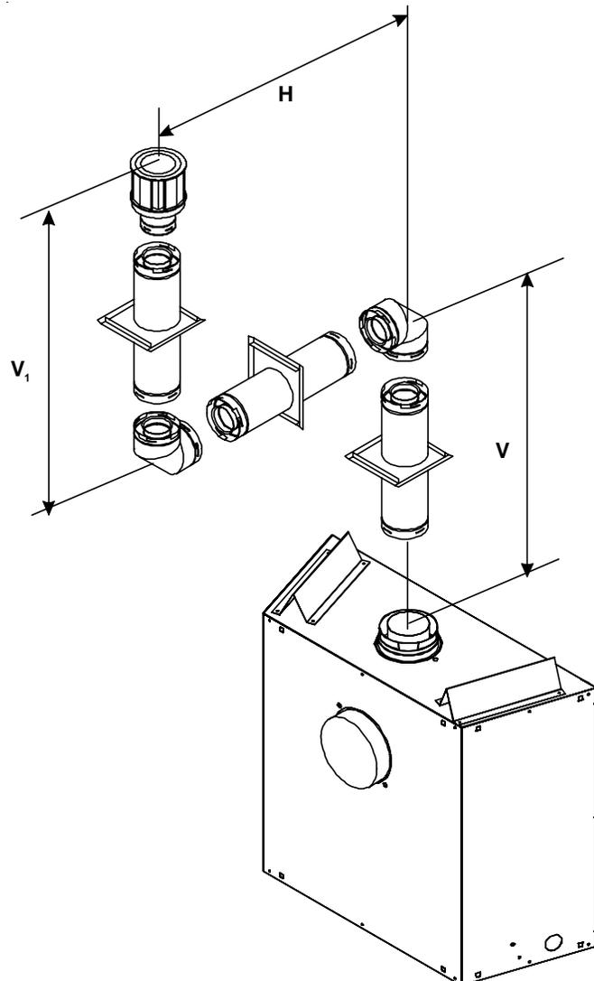
**NOTE:** There **MUST** be a 25% reduction in total H when using flex vent except when using the simple up and out installation (see Figure 9).
