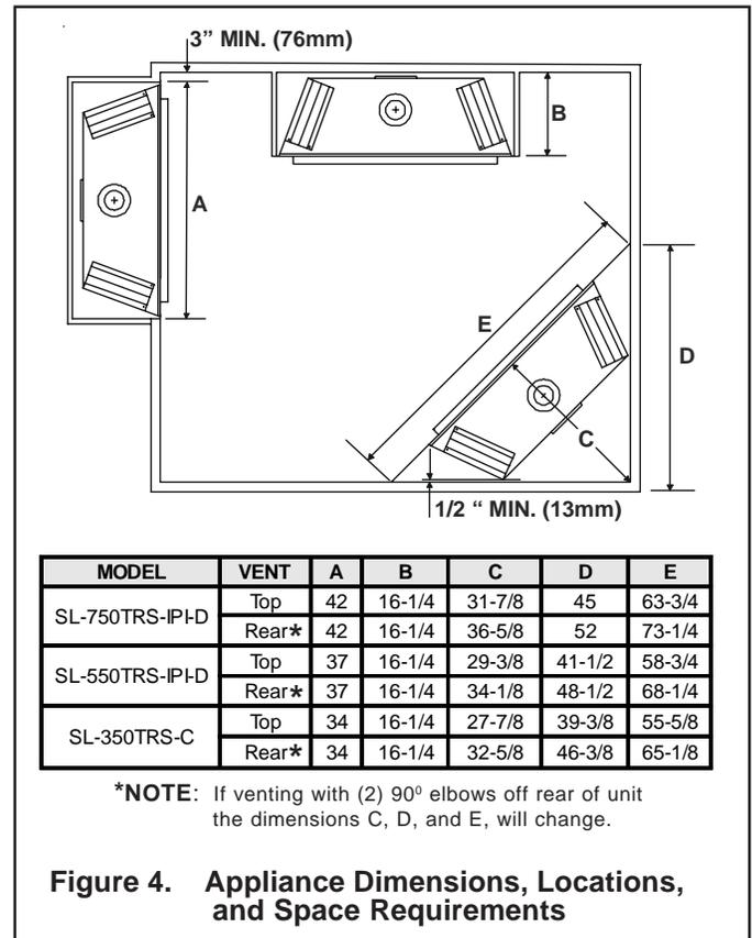
**Figure 4. Appliance Dimensions, Locations, and Space Requirements**
