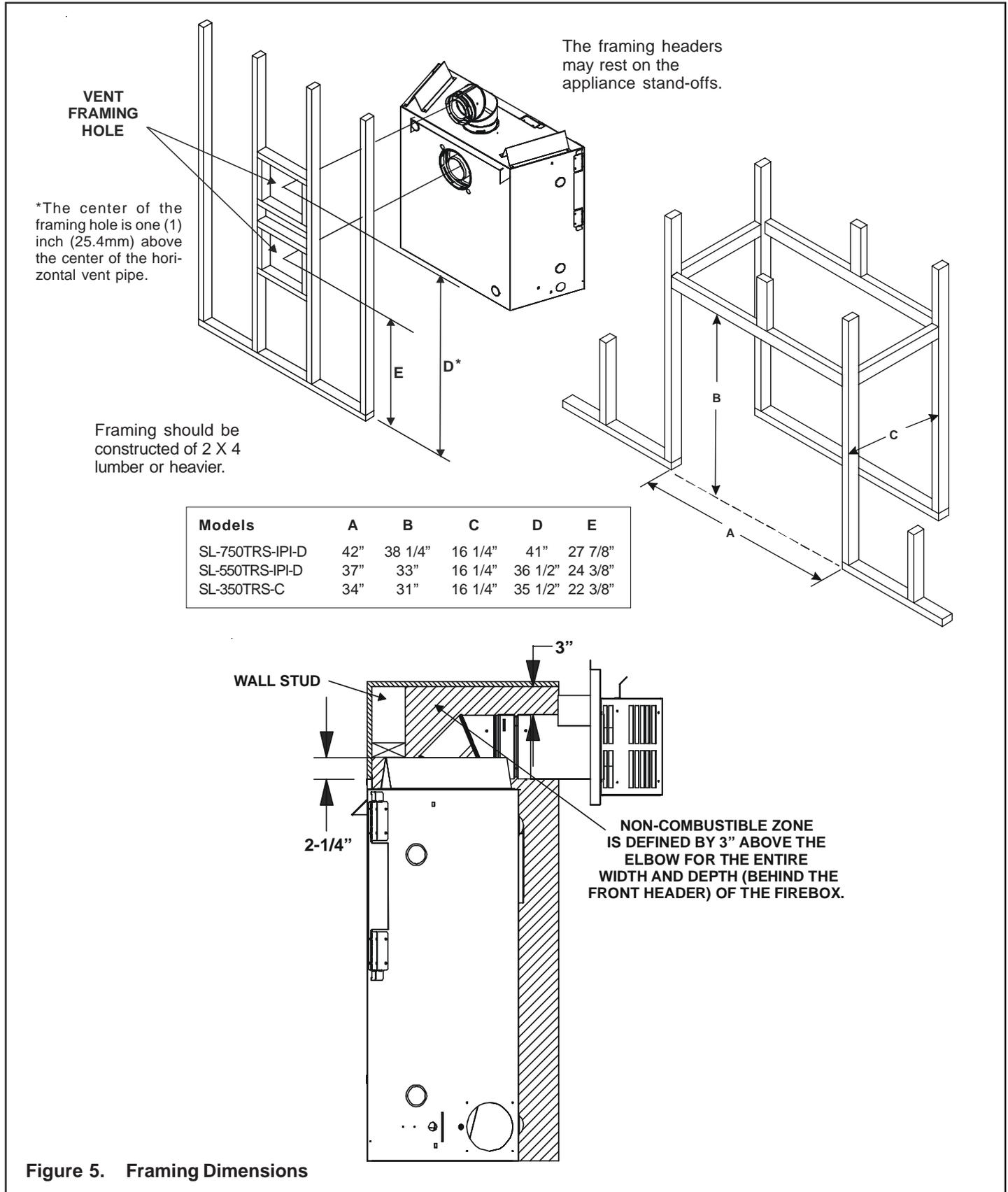
Figure 5. Framing Dimensions
