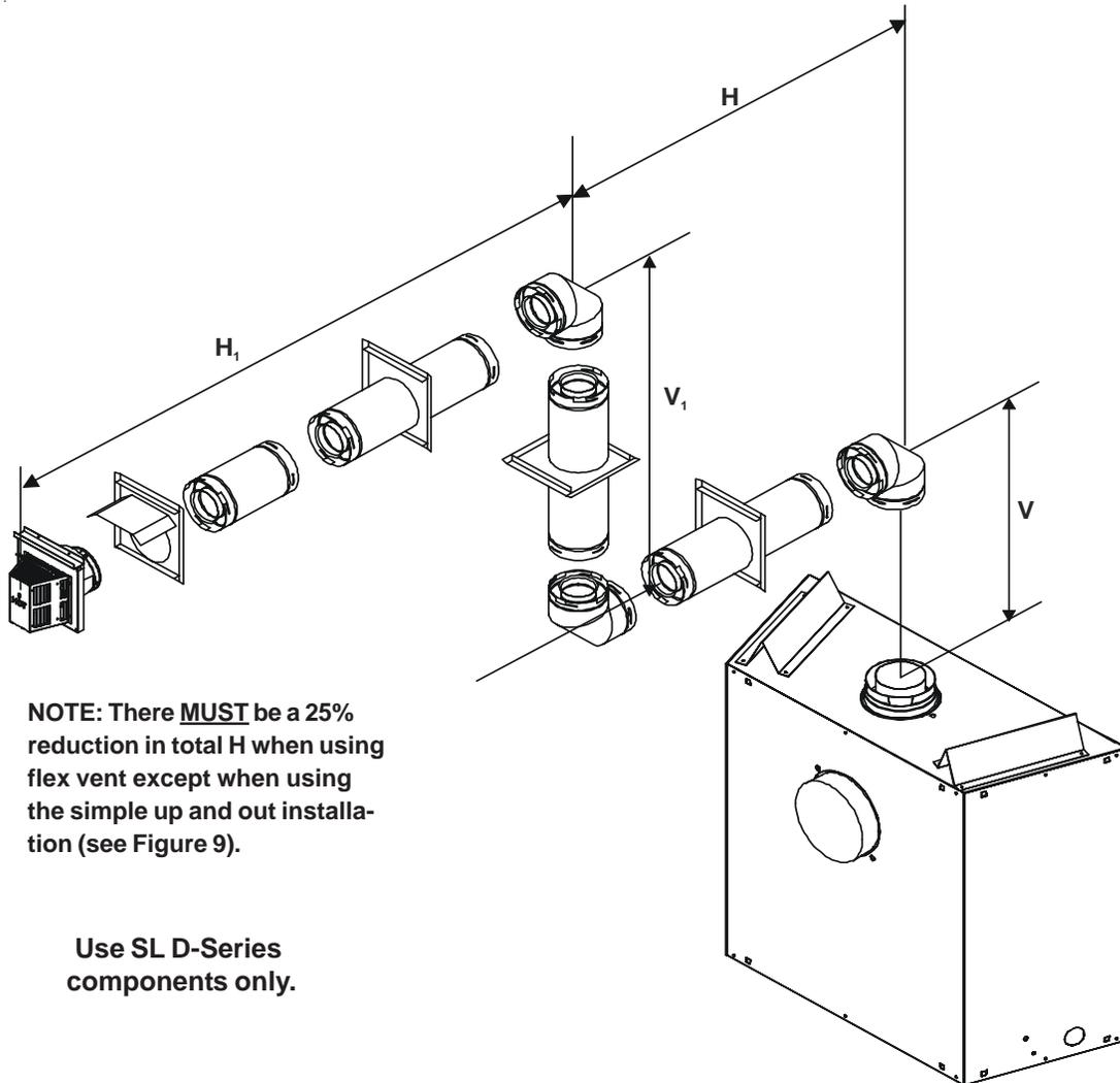
**NOTE:** There MUST be a 25% reduction in total H when using flex vent except when using the simple up and out installation (see Figure 9).
