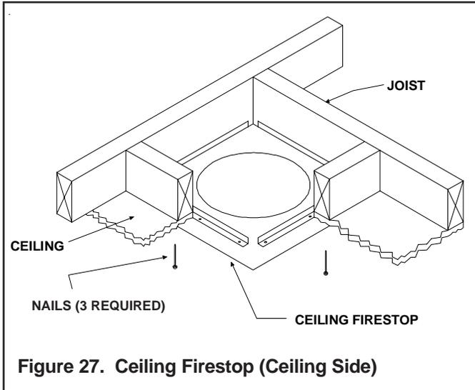
**Figure 27. Ceiling Firestop (Ceiling Side)**
