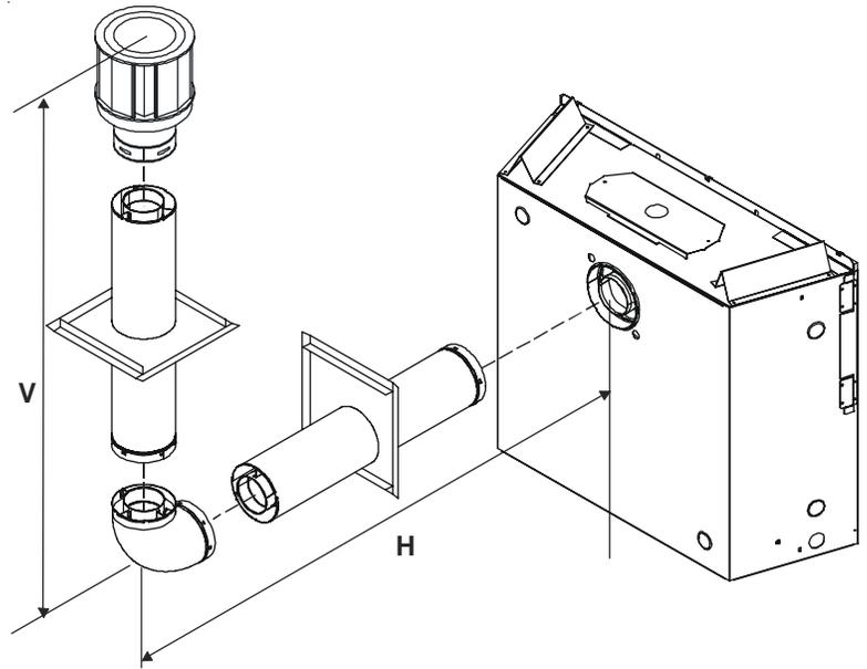
Figure 12. Venting with One 90° Elbow
