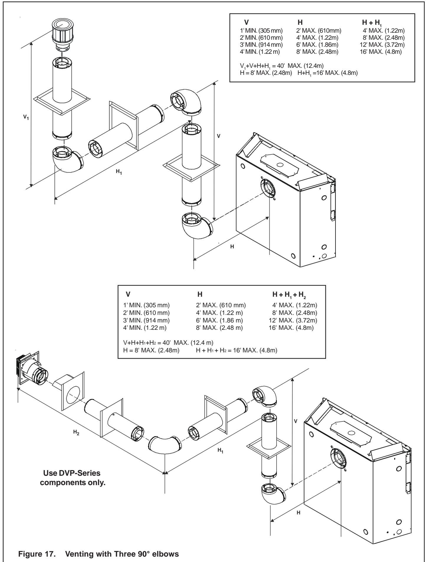
**Figure 17. Venting with Three 90° elbows**
