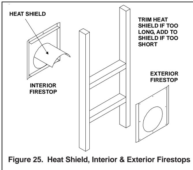
**Figure 25. Heat Shield, Interior & Exterior Firestops**
