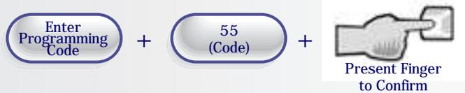
Note: If programming code is lost, Remove the Tamper Wing and hold down the 5 key during power-up and enter the default programming code '6666'.
