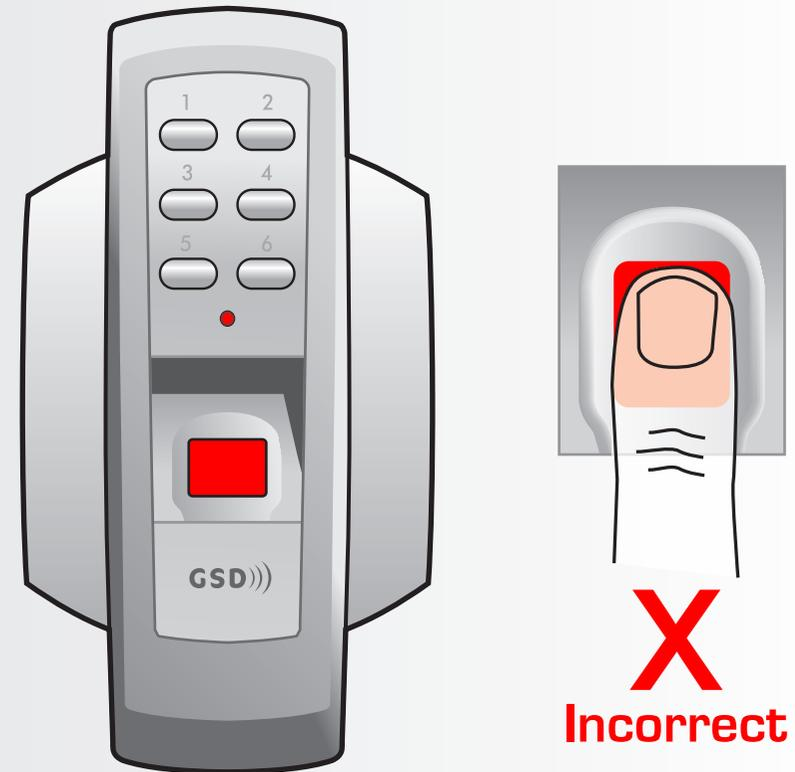
**Note:** Incorrect placement : finger does not fully cover the sensor window. The door control will not respond and the red light will not turn off if the sensor window is not fully covered by the finger.
